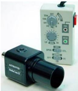
The Stellacam II system is monochrome (detects only black and white) and are said to produce greater details. A high resolution black and white monitor is recommended; however almost any TV monitor with a video in jack will work. Monitors ranging in size from 8” to 12” provide very pleasing views. A 12” monitor seems to be the choice among video observers. For public events some imaginative observers are using big screen TVs in the back of vans and SUVs to create mini observatories.
