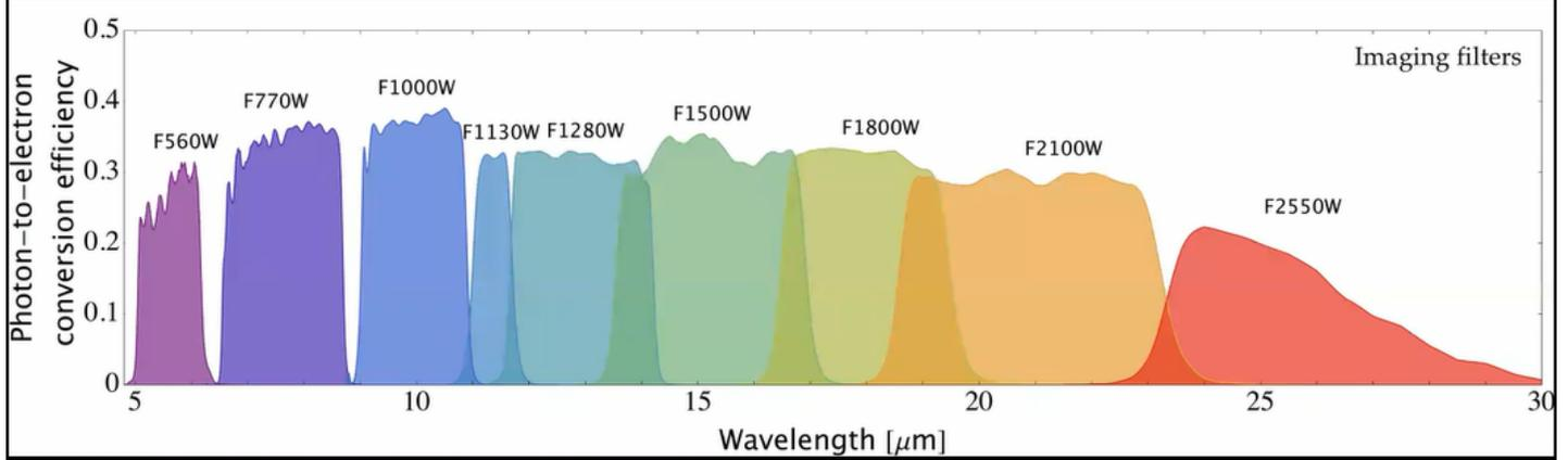
Imaging & spectroscopy bandpass diagrams for the JWST Mid InfraRed Instrument (MIRI)
