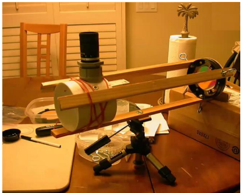
National Geographic 3” reflector, rebuilt as a travel telescope
